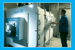
The flow characteristics of the Filterfans 4.0™ were optimized during more than 1,000 tests in our modern test laboratory. The result: modern louvers which enable maximal airflow, hold back dust and water particles, protect the filter medium from damage and can be integrated into the design of the applications.
