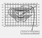
Mounting Height: 25' (7.6m) A.F.G Initial Delivered Lumens: 25,000 Initial FC at grade
