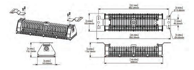
C) For wall mounting, the BL-WM kit is required. Install wall mounting brackets on the BL luminaire as shown using the provided M6 fasteners. Torque M6 fasteners to 4.5 N-m [40 in-lbs]. Mount fixture to desired location using  $4x \frac{1}{4}$ -20 or M6 fasteners.
