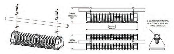
G) For strap mounting onto structural elements, install supplied straps through the slots at the ends of the luminaire and around mounting point. Feed open end through worm drive and tighten screw to secure luminaire.
