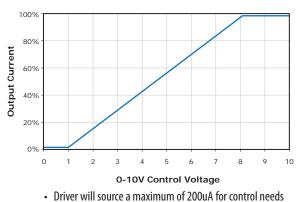
Controller must sink current from the 0-10V control leads
