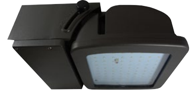
AD25Q Shown with "AD25WB" Wall Mount Box, Die-Cast Wall Mount box, Allows Housing to Swivel 0° Up to 30°, Bronze Powdercoat Finish. Twist-Lock Photocell Option Not Available with this Mounting.
