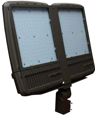
KH45Q Shown with "LSF, TM" External Mount Slipfitter & Twin Mount Assembly, External Mount Die-Cast Adjustable Slipfitter for 2 3/8" Tenons, Bronze Powdercoat Finish, Includes Hardware.
