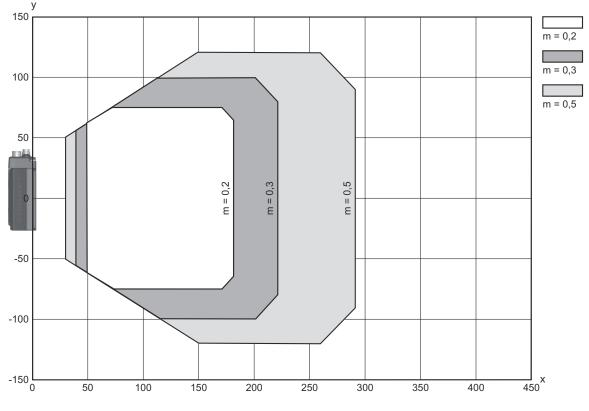
Х Reading field distance [mm]
