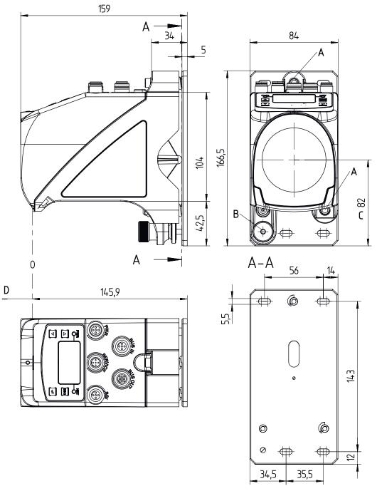
А M5 screw for alignment C Optical axis
