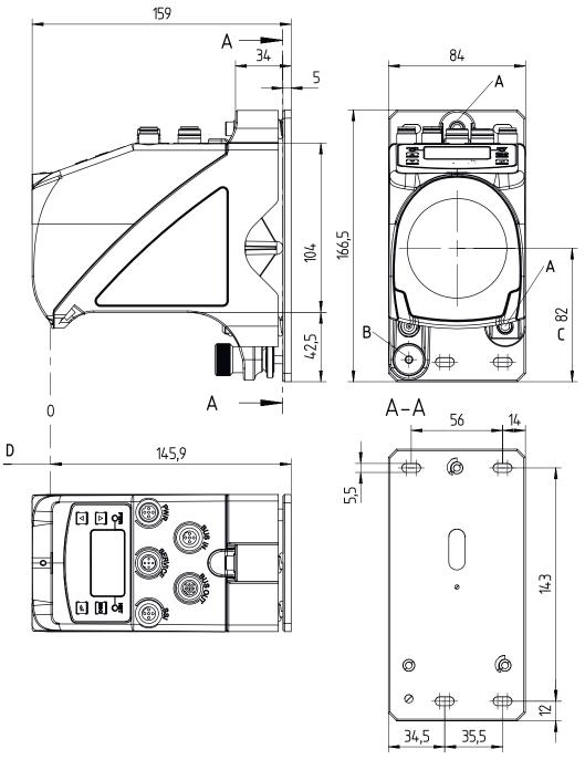
A M5 screw for alignment
