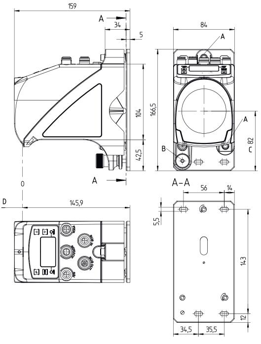
A M5 screw for alignment
