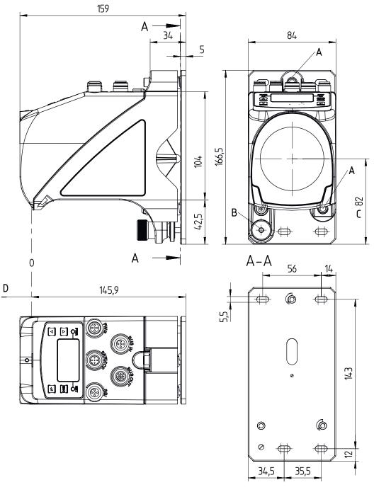
A M5 screw for alignmentB Knurled nut with WAF4 h
