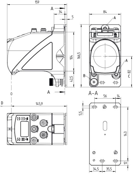
A M5 screw for alignment
