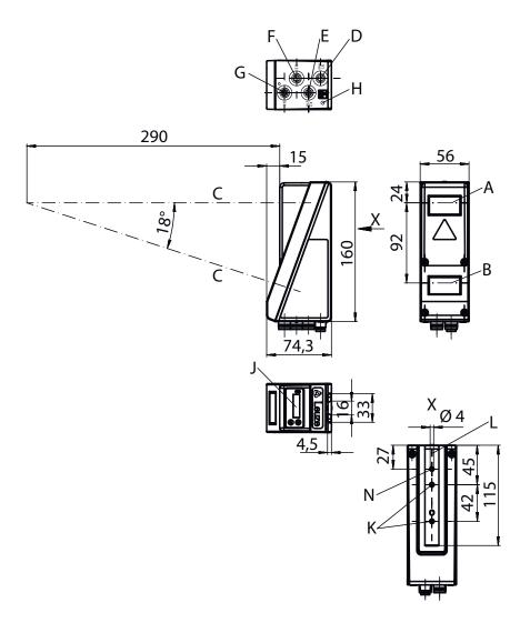
Transmitter Receiver Optical axis D, E, F, G X1-X4 connections
