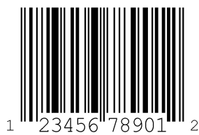
Figure 17.3: Code type 06: UPC-A
