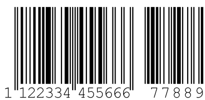
Figure 17.6: Code type 10: EAN 13 Add-on
