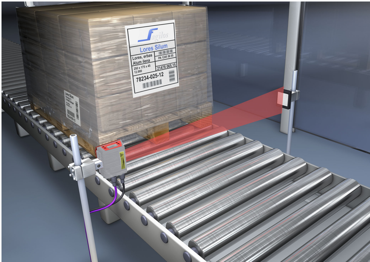
Figure 4.2: Reflector arrangement for autoReflAct
