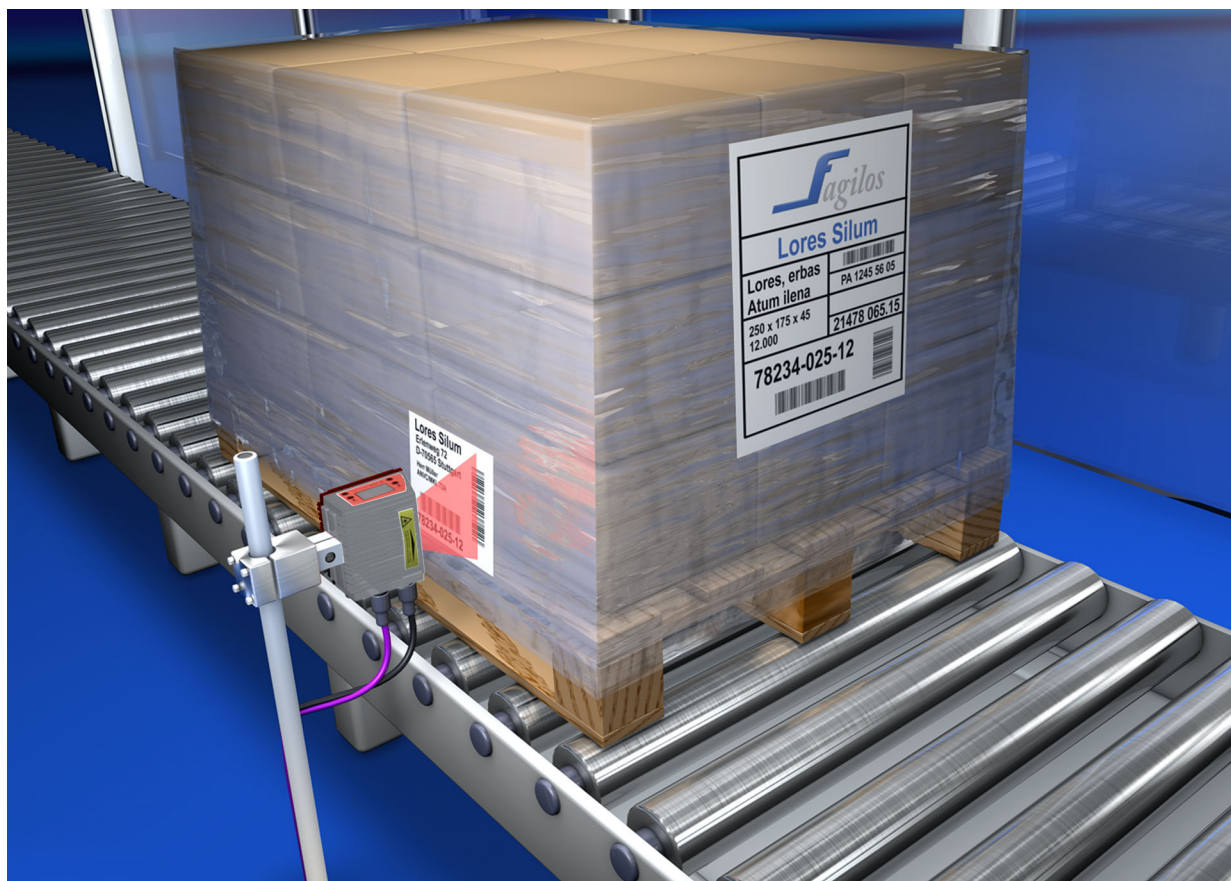
Figure 5.1: Deflection principle for the line scanner
