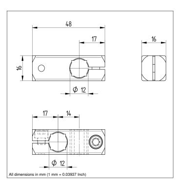
The mounting clamps function as a connection technology and can be clamped onto mounting profiles and/or rods.
