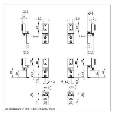
Suitable for lateral mounting of SEFGxxx and SEMGxxx safety light curtains, SEFBxxx safety light arrays and OSElxxx and OEElxxx light curtains for measuring tasks on aluminum profiles or walls. The mounted sensors can be installed rotated by  $\pm 15\,^\circ$  depending on the application.
